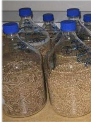
Figure 3: Storage experiments for pellets in 5-liter glass bottles
