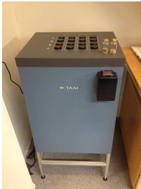
Figure 4: The eight channel TAM Air 3116-2 isothermal calorimeter
