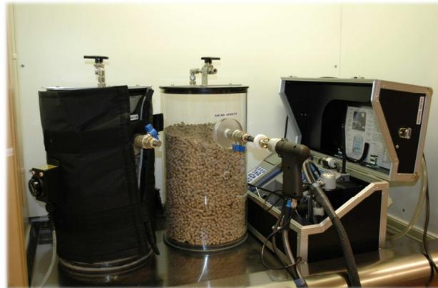
Figure 2: Setup for measuring the off-gassing of CO, CO<sub>2</sub> and CH<sub>4</sub>.
