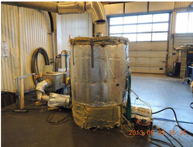
Figure 18: Photo of the 1 m 3 test set-up with the insulated test container
